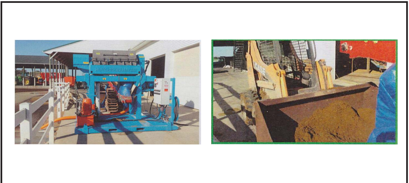
Figure 4. A centrifuge to precipitate manure solid rich in P (left) and manure solid after centrifuging (right); pictures used with permission.
